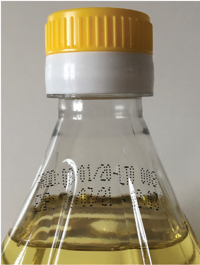
Figure 4.17 Date marking on a bottle printed using the dot matrix printing concept.
